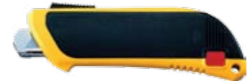
Flex Guard Safety Knife ● OS-SK-6 Automatic protection system engages when the blade loses contact with the cutting surface. Built-in safety protection is activated as soon as you start cutting and cannot be overridden. Rounded Safety Tip Blades further reduce the possibility of injury. For left-handed or right-handed users. Cuts to a depth of 0.39" (10mm). Uses OS-RSKB-2/10B and OS-RSKB-2/50B replacement blades.
